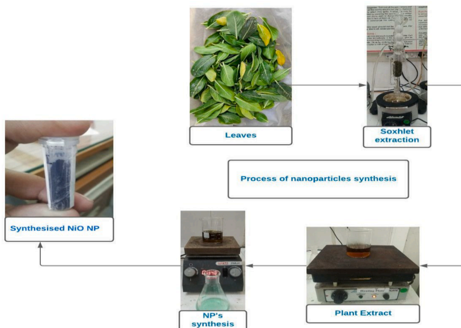
Fig. 3. Mechanism of the plant mediated synthesis of NiO NPs (Barzinjy et al., 2020; Imran Din and Rani, 2016).
